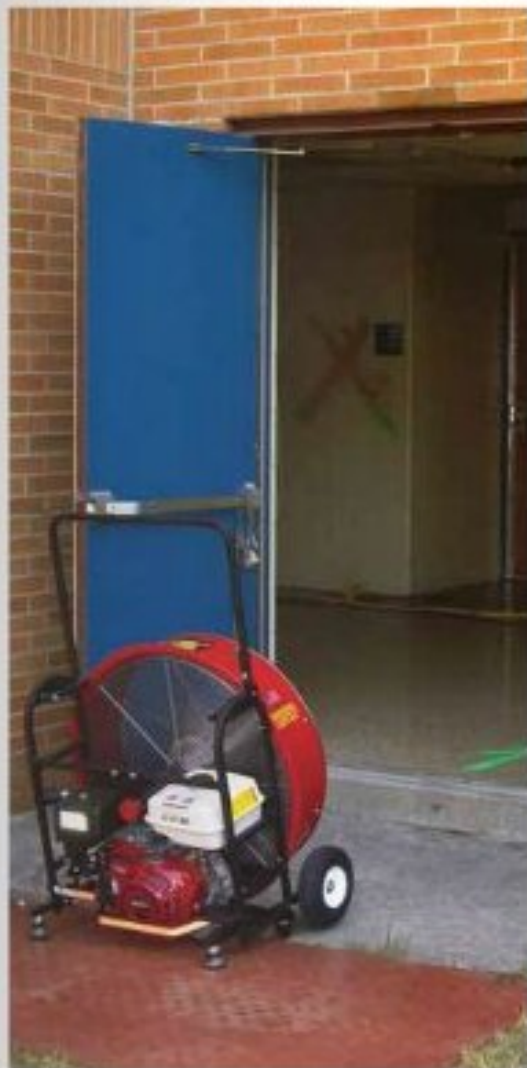
Fan placed at an entrance of a high-rise building. Picture courtesy of Tempest Technology Corporation
